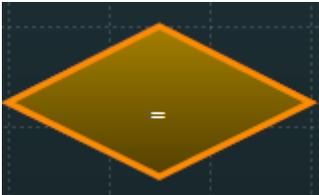
contains the condition that will have to be verified. From a Condition object can exit a “Yes” link, which will be connected to the action to take if the condition is verified, or a “No” link, which will be connected to the action to take if the condition is not verified.
